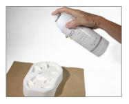
4. Hold the can of **MO-RE** at a 45° angle, 10-14 inches from the mold.
