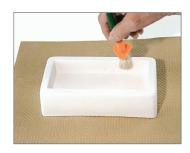
1. Using a nylon brush, gently sweep any loose powder from the cavity of the mold.
