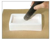
2. Vacuum the dust with your studio Shop Vac. (NOTE: A HEPA filter is always recommended when vacuuming
